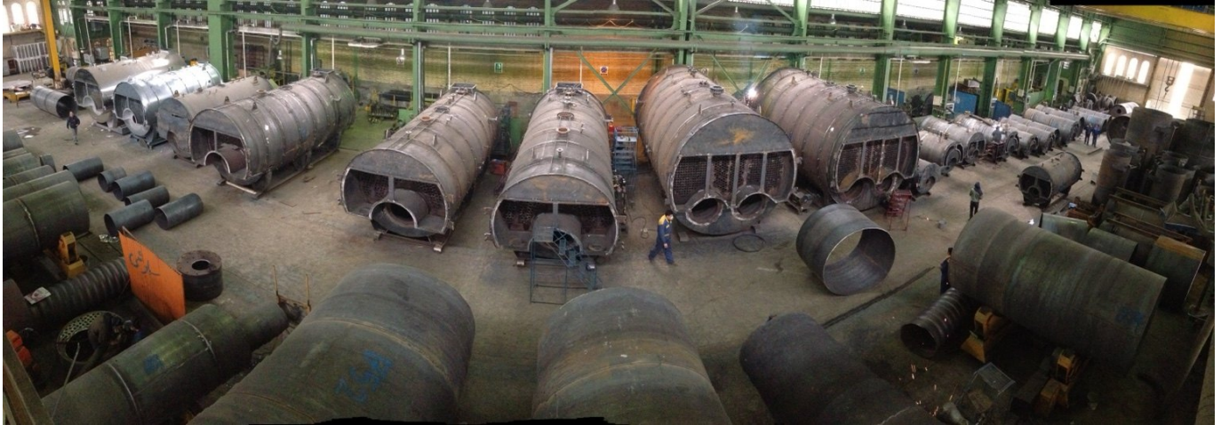
Production hall: boiler shells and assemblies at different stages of manufacture.
