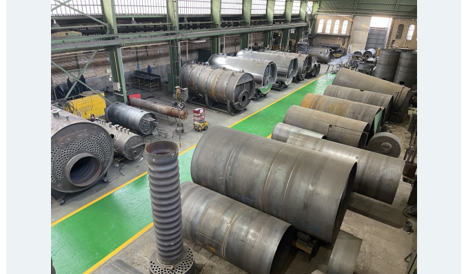
Boiler shells and components in fabrication
